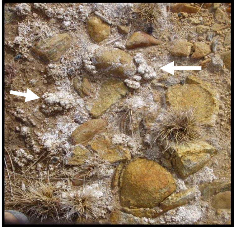
Figure 10. The mineral aluminite is shown here as sulfate “blooms” (white arrows) associated with iron-stained cobbles within the riverbed. This is a diagnostic indicator of the presence of sulfate-saturated ground waters. The sulfate originates from acidic ground water created by sulfide decomposition and it permeates the tailings-impacted portion of the river floodplain.
